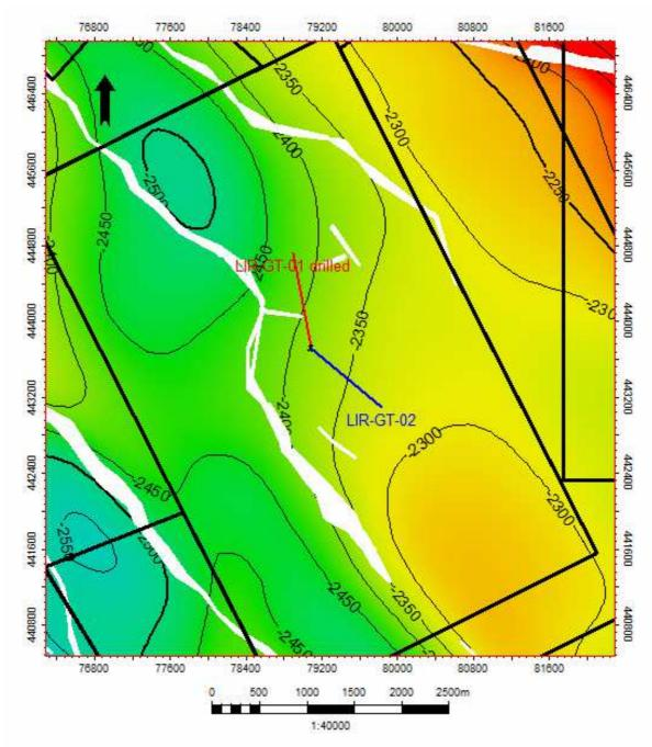
Fig. 6 – Top Structure map with well trajectories of LIR-GT-01 (drilled) and LIR-GT-02 (planned)
